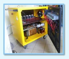
material. Post Weld Heat Treatment, or Stress-relieving as it is commonly called, significantly reduces the stresses and improves the hardness and ductility of the material.
